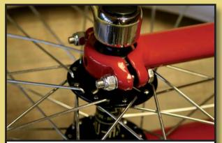
TIGHTEN BOTH SCREWS EVENLY SO THAT DISTANCE BETWEEN FRAME & CUPHOLDER IS THE SAME ON BOTH SIDES. BUT NOT TOO TIGHT!
