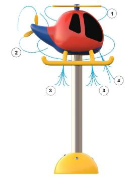
The helicopter is equipped with four push buttons in the half sphere. The displayed water effects and rotation of the blades are initiated by the buttons.
