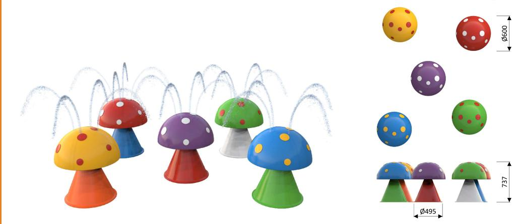
Including: control unit and 4 valves Please note that the installation of the control unit will *not* be done by Aqua Drolics Water connection Water consumption Water pressure Max. waterdepth Mounting Place of spout nozzles Suitable for 5 x Ø32 mm (PVC DN 25) 5 m<sup>3</sup>/h 0,6 - 1 bar 300 mm Aqua Drolics System D On top of the mushrooms Toddlers and children
