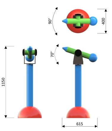
Water connection Water consumption Water pressure Max. waterdepth Mounting Place of spout nozzles Suitable for Ø32 mm (PVC DN 25) 1,5 m³/h 0,6 - 1 bar 350 mm Aqua Drolics System B + D Front side of the shooter Toddlers, children, youth
