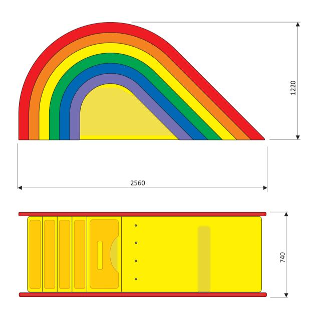
The rainbow slide can be placed in a pool as well as over a pool's edge. If there is a water supply the slide can spout water from the surface. Adjustments can be made on request.
