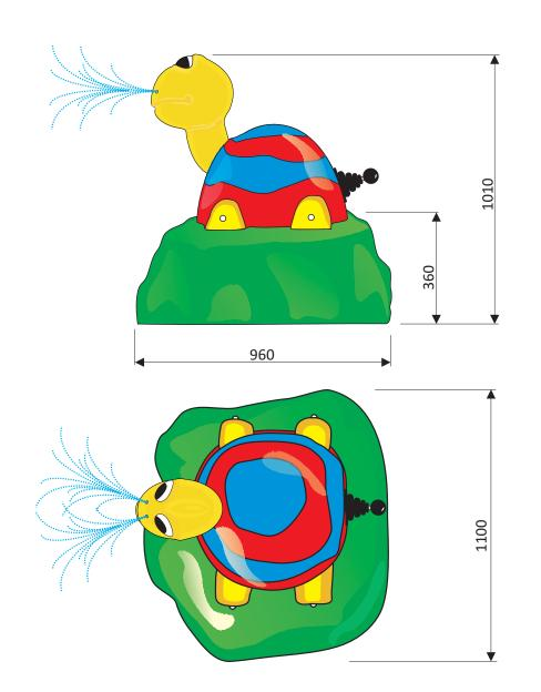
The turtle has a built in hand pump. The turtle is also available as a spouting object without hand pump (8929b). By moving the handle the turtle spouts water from its nose.
