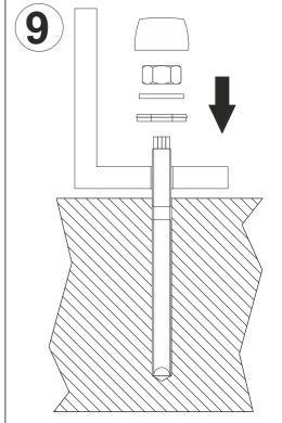
Mount the product. If necessary, shorten the anchor shaft using the hacksaw.
