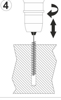
Brush the holes using the steel brush (Ø 11 mm).
