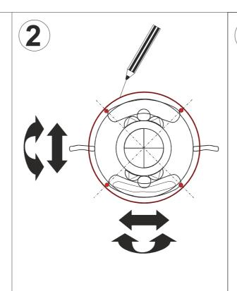
Determine the position of the product. Mark the outline and position of the holes on the sub-soil.
