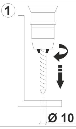
Drill 4 holes  $\varnothing$  10 in the product flange, as shown in the products drawing.
