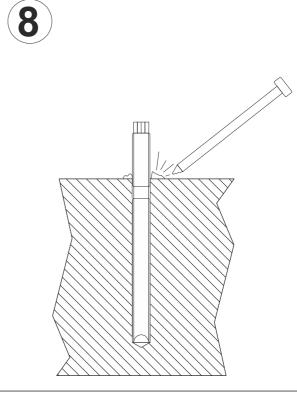
Remove any remains around the anchor shaft.
