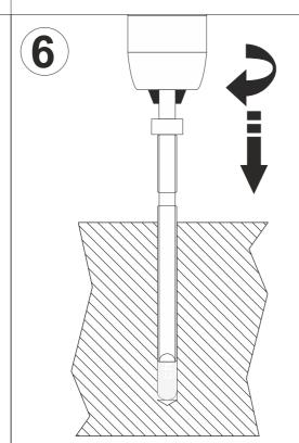
Place anchor shaft using the delivered tool.
