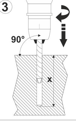
Drill holes in the sub-soil using the concrete drill. Depth as shown in the products drawing.
