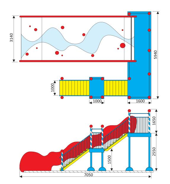
The family slide can be fixed in the pool or at the pool's surround. By fixation at the pool's edge, the water depth has to be at least 1000 mm. Adjustments can be made on request.
