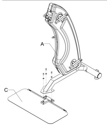
Firstly, take off the screws and washers from the base bard set (C) and then install the base bard set (C) to the main frame set (A); secondly, fix with the screws and washers taken before.
