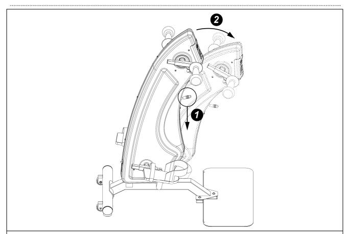
According to the order in the figure, **1** press the driving lever of the gas spring downward;
