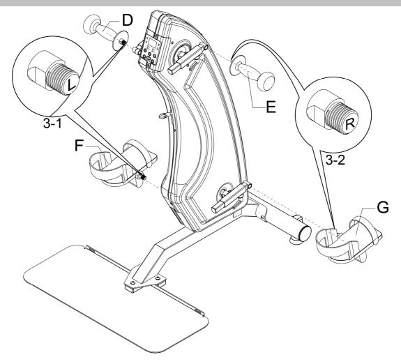
Follow the image, lock the left and right handrail sets (D  $\cdot$  E) and the left and right pedal (F  $\cdot$  G) with opening wrench, then fix to the main frame set (A).
