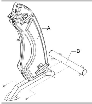
Firstly, take off the screws on the front stabilizer, and then place the front stabilizer tube (B) to the main frame set (A), and lock with the screws taken off before.
