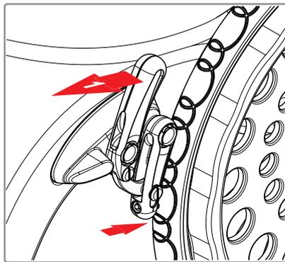
**-Do not use the brakes to stop the wheelchair in movement**
