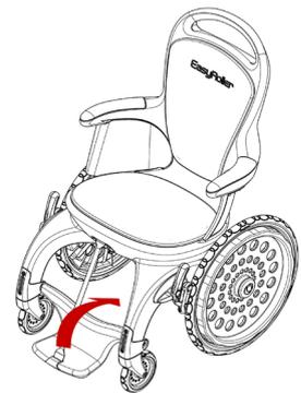
Normally, when getting out of the wheelchair the footrest is tilted up. The footrest is designed that one does not need to tilt it up when one wants to exit the chair. Place simply your feet's on the outside of the footrest when you want to get up.
