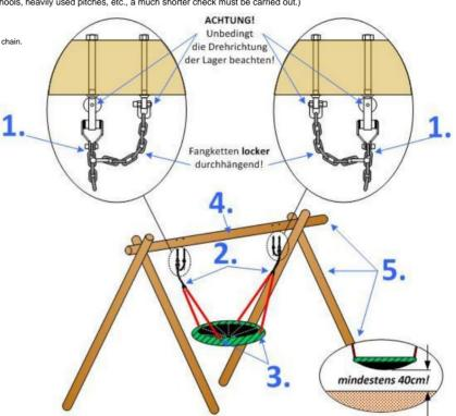
Observe the rotation and installation direction according to the drawing above (here for a bird's nest 1.20 m Ø with internally mounted safety bearings) When assembling the mini bird nest and the honeycomb nest, the catch bearings must be mounted on the outside!
