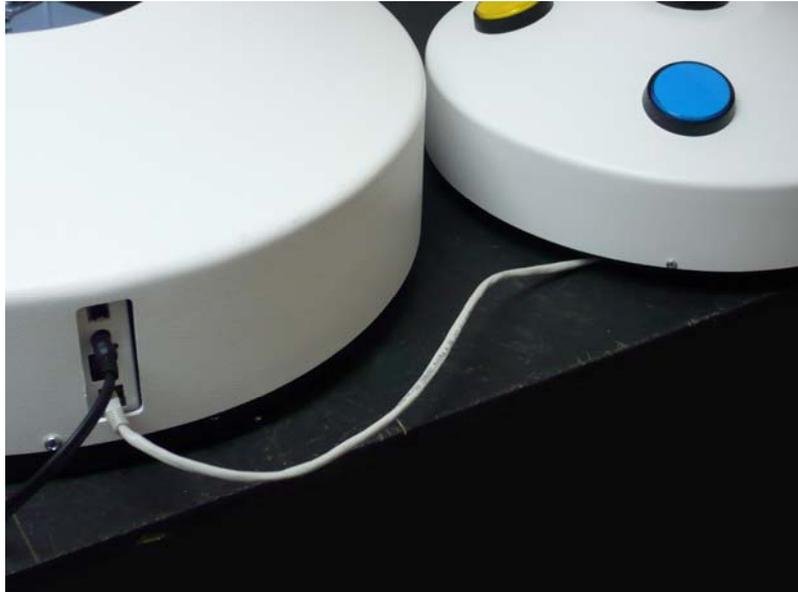
Switch off the Bubble Tube completely. Connect the 5 Button Switch Box (A) to the base of the Bubble Tube (J).
