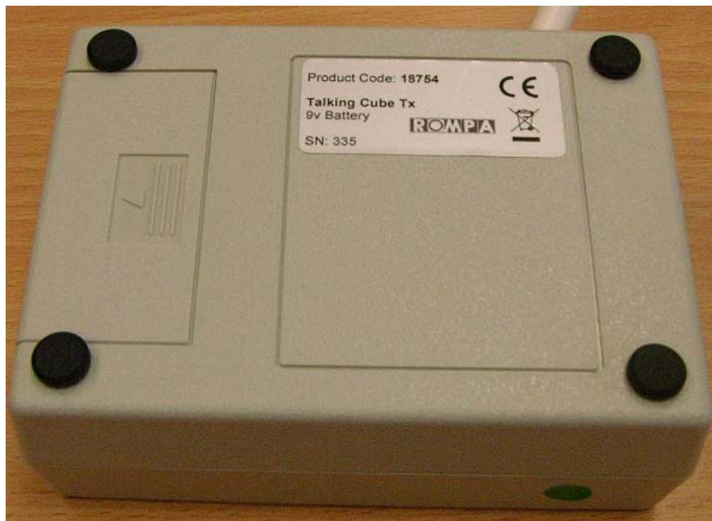
Remove the exhausted battery and replace with a new battery of the same specification. Do not attempt to access the interior of this box. Push the grey box back into the Talking Cube and close the zip. ***Make sure the grey box is put back in the correct way round – coloured stickers indicate the correct orientation.***
