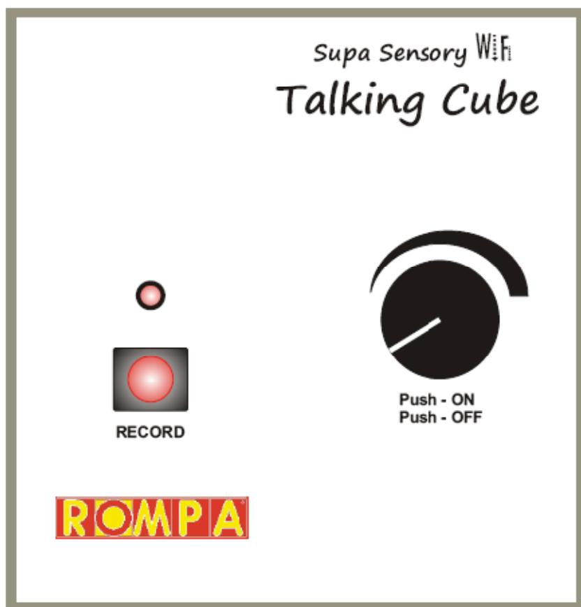
3. Make sure the switch on the cube itself is ON. It is switched ON when the switch shows RED. The Talking Cube is supplied with a pre-recorded message on each side. To change this recording, place the cube so that the side you wish to associate a message to is facing upwards.
