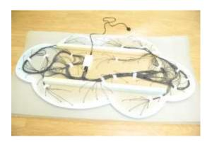
4. Screw the 4 eyelets firmly into the 2 wooden bars that go down the length of the Cloud. We cannot be specific where to put these as it will depend on where you wish to attach them to the ceiling, but try to put them towards the four corners so it hangs evenly.
