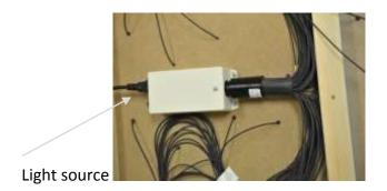
9. Make sure the cable is out of reach and will not be pulled - conceal the cable behind trunking for example as required.
