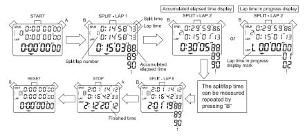
**Note:** 1. When the number of stored measurements exceeds 90, flashing "FULL" appears, and when it exceeds 100, a warning sound start beeping.
